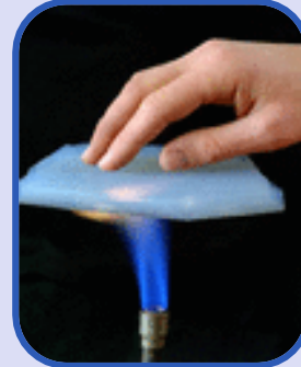
Aerogel produced from silica, sometimes called frozen smoke
